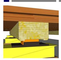
KTL SPORT PRO II is an area-elastic sports floor, based on 22mm solid hardwood 2-strip parquet boards, nailed to a resilient 1-layer batten system, installed and levelled over concrete subfloor. Total construction height excluding packing is 64mm.
