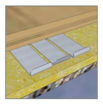
KTL SPORT PORTABLE PRO SYSTEM is an area-elastic sports floor, based on 22mm solid hardwood 8-strip or multi-strip panels, laid floating in a brick pattern on an existing sports floor or on levelled concrete. The panels connect to each other on all sides by means of the unique flexi-lock system. The panels come with a supporting 12mm plywood underlay. Total construction height including KTL 10mm sports foam is 44mm.
