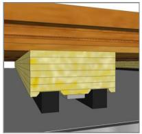
KTL SPORT PRO I is an area-elastic sports floor, based on 22mm solid hardwood 2-strip parquet boards, nailed to a resilient 1-layer batten system, installed floating on levelled concrete or wooden based subfloor. Total construction height including the floor board is 50mm.
