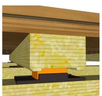
KTL SPORT PRO II - 2 LAYER SYSTEM is an area-elastic sports floor, based on 22mm solid hardwood 2-strip parquet boards, nailed to the resilient 1-layer PRO II batten system, which is installed onto un-elastic under battens, levelled over concrete subfloor. Total construction height, excluding packing material is 136 mm. Can be raised to 250mm.
