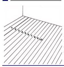
The boards are nailed to the battens in accordance with a 10-board measurement, allowing the boards to expand and contract with the fluctuation in the climatic conditions within the building. The 10 board measurement is specified on the basis of the expected maximum relative humidity level in the building when in use - and tells how much 10 boards must cover, when installed.
