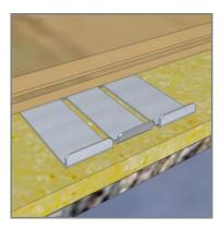
KTL SPORT PORTABLE PRO SUMMIT SYSTEM is an area-elastic sports floor, based on 22mm solid hardwood 8-strip or multi-strip panels, laid floating in a brick pattern on an existing sports floor or on levelled concrete. The panels connect to each other on all sides by means of the unique flexi-lock system. The panels come with a supporting full plywood underlay. Total construction height including KTL 10mm sports foam strips is 44mm including full 12mm plywood layer.
