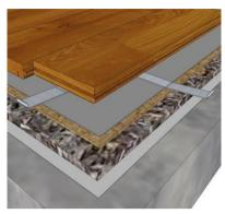
KTL SPORT MULTI CLIP is an area-elastic sports floor, based on 22mm solid hardwood 2-strip parquet boards connected with clips, including clips at board ends, and installed floating over foam and possible load distribution sheets, on levelled concrete or wooden based subfloor. Total construction height including the floor board is 32mm to 40mm, depending on the elastic underlay chosen.
