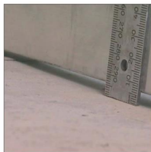
Subfloor flatness needs to be within the required tolerance
